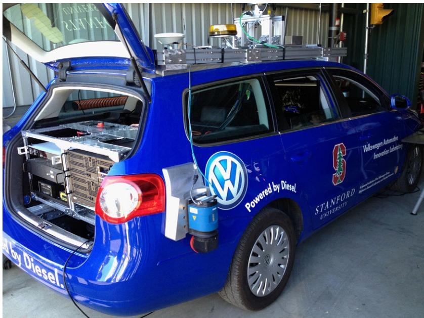
*‘Junior’, one of Stanford University’s bespoke test vehicles capable of fully-autonomous operation. (Photo by S Le Vine July 2013)*
