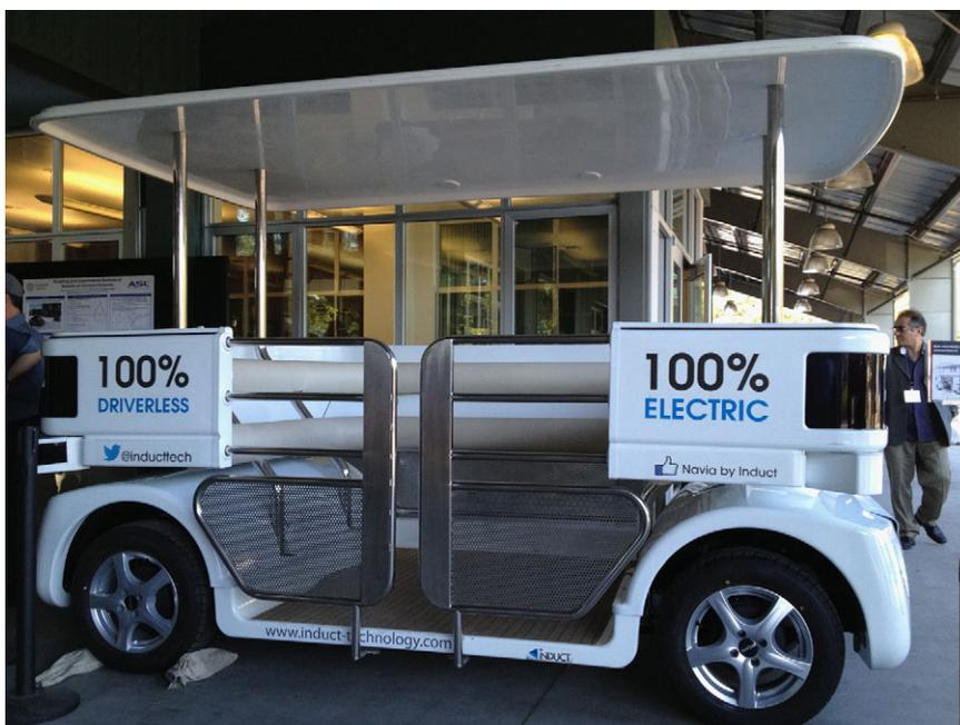
A driverless shuttle vehicle designed for light-traffic public transport service, CityMobil2 EU-supported research project (Photo by S Le Vine July 2013)
